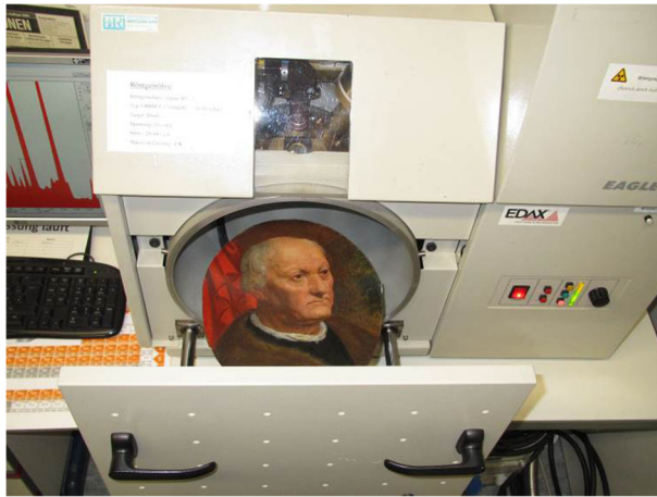
Fig. 6 The analyzed artwork “Bildnis eines jüdischen Kaufmans”, in situ in the opened large measurement chamber of \mu -XRF (Eagle II)
