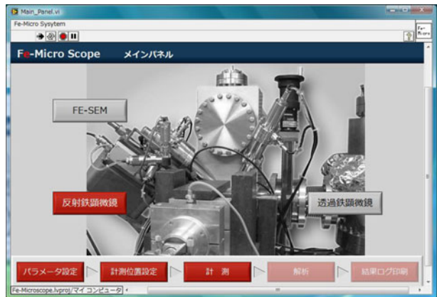
Fig. 1 Main panel of the LabVIEW operating system for Mössbauer spectroscopic microscopy
