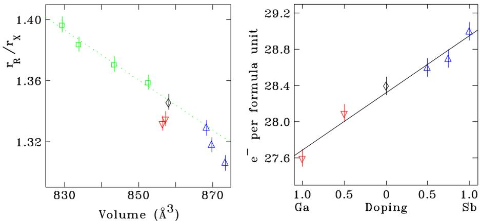
**Fig. 2** (Left) Cell volume dependence of the atomic radii ratio ( $r_R/r_X$ ).  $\square$  (green) and the dashed line show the trend for  $\text{Yb}_5\text{Ge}_{4-x}\text{Si}_x$  [4].  $\nabla$  (red) and  $\triangle$  (blue) show data for gallium and antimony doping respectively. (Right) Dopant dependence of the weighted valence electron count
