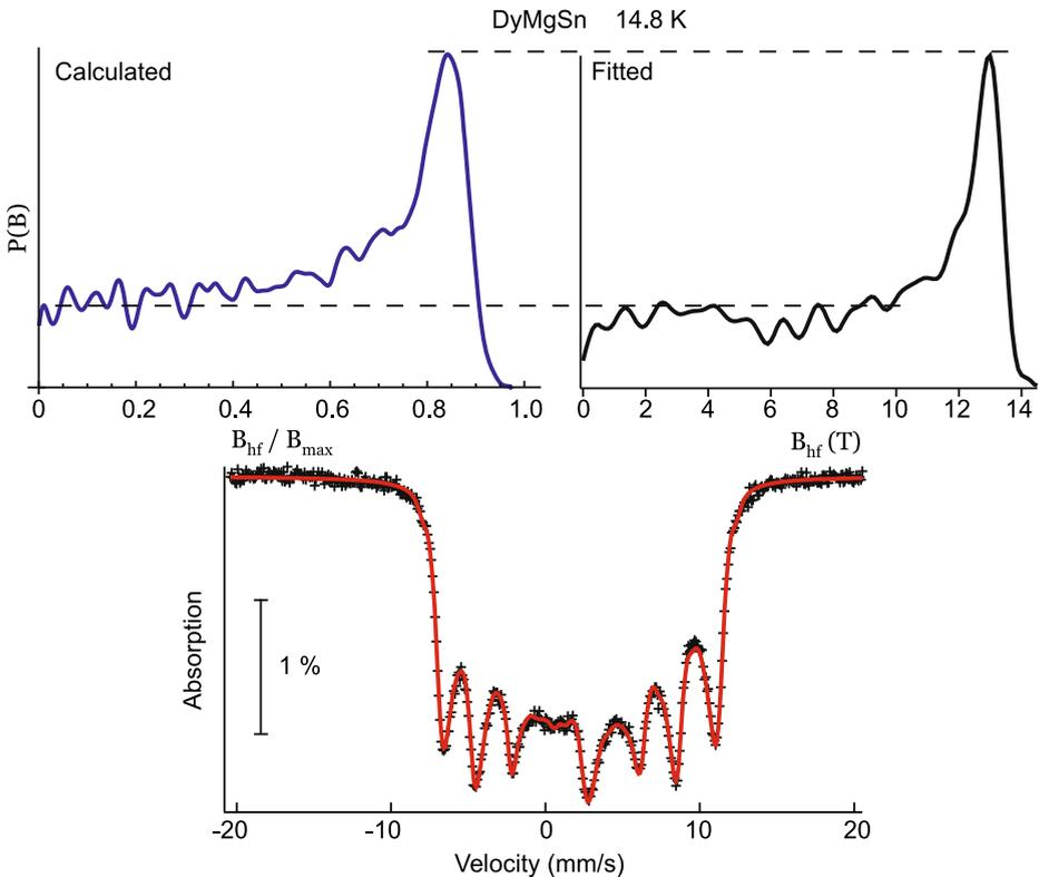
**Fig. 6** Top left Calculated THFD assuming a sine-wave modulated magnetic structure as described in the text. Top right Fitted THFD of DyMgSn obtained from the  $^{119}\text{Sn}$  Mössbauer spectrum of DyMgSn at 14.8 K. The dashed lines emphasise that the plateau height is the same in both patterns. Bottom:  $^{119}\text{Sn}$  Mössbauer spectrum of DyMgSn at 14.8 K and fit to the data (solid red line)
