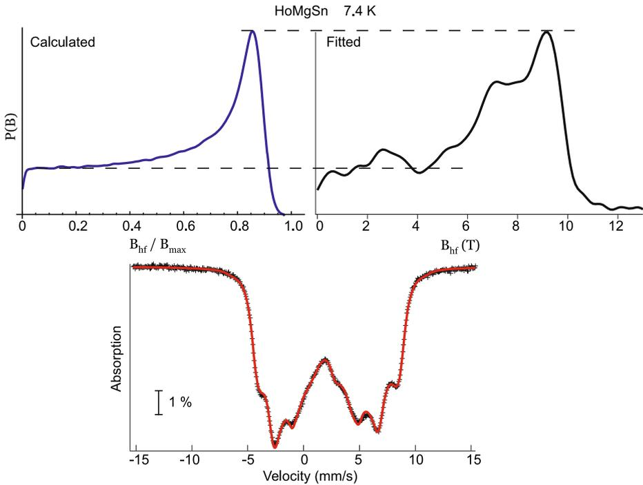
**Fig. 3** *Top left* Calculated THFD assuming a magnetic structure showing the first and third harmonics of the  $\mathbf{k}$ -vector as described in the text. *Top right* Fitted THFD of HoMgSn obtained from the  $^{119}\text{Sn}$  Mössbauer spectrum of HoMgSn at 7.4 K. The *dashed lines* emphasise that the plateau height is the same in the calculated and fitted patterns. *Bottom*  $^{119}\text{Sn}$  Mössbauer spectrum of HoMgSn at 7.4 K and fit to the data (*solid red line*)
