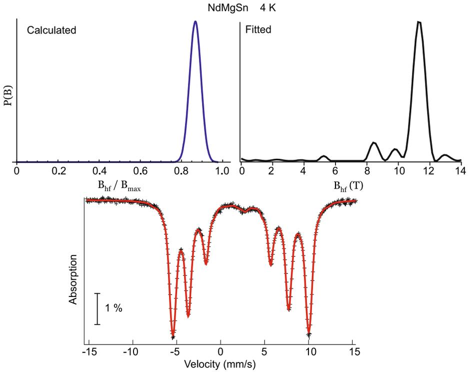
**Fig. 2** *Top left* Calculated THFD assuming a commensurate antiferromagnetic structure. *Top right* Fitted THFD of NdMgSn obtained from the  $^{119}\text{Sn}$  Mössbauer spectrum of NdMgSn at 4 K. *Bottom*  $^{119}\text{Sn}$  Mössbauer spectrum of NdMgSn at 4 K and fit to the data (solid red line)
