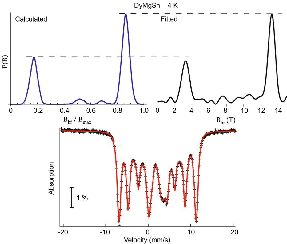
**Fig. 5** *Top left* Calculated THFD assuming a square-wave modulated magnetic structure as described in the text. *Top right* Fitted THFD of DyMgSn obtained from the  $^{119}\text{Sn}$  Mössbauer spectrum of DyMgSn at 4 K. The dashed lines emphasise that the peak heights are the same in the calculated and fitted patterns. *Bottom*  $^{119}\text{Sn}$  Mössbauer spectrum of DyMgSn at 4 K and fit to the data (*solid red line*)
