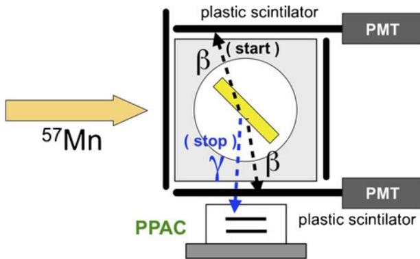
**Fig. 1** Experimental layout of the  $\beta - \gamma$  coincidence measurement of in-beam Mössbauer spectra of  $^{57}\text{Fe}$  using  $^{57}\text{Mn}$  implantation
