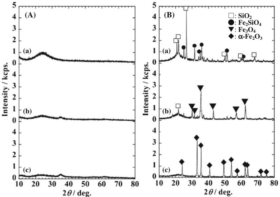
**Fig. 2** XRD patterns of  $x\text{Fe}_2\text{O}_3 \cdot (100-x)\text{SiO}_2$  glass with 'x' of **a** 10, **b** 30 and **c** 50 measured **(A)** before and **(B)** after annealing at  $1000^\circ\text{C}$  for 3 h
