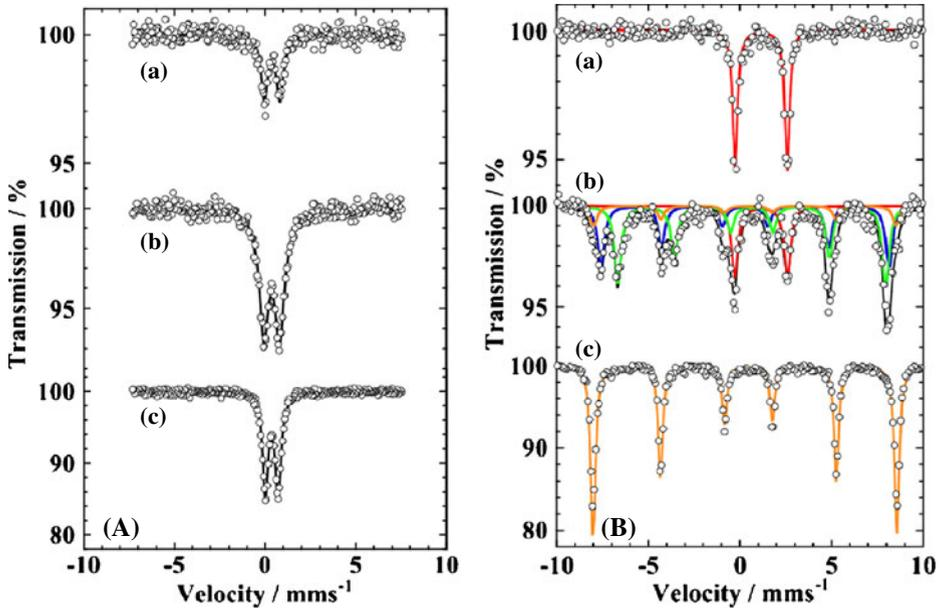
**Fig. 1**  $^{57}\text{Fe}$ -Mössbauer spectra of  $x\text{Fe}_2\text{O}_3 \cdot (100-x)\text{SiO}_2$  glass with ‘ $x$ ’ of **a** 10, **b** 30 and **c** 50 measured **(A)** before and **(B)** after annealing at  $1000\text{ }^\circ\text{C}$  for 3 h
