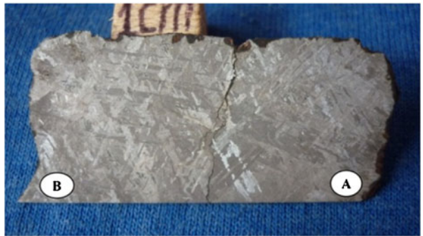
Fig. 2 Widmanstätten pattern of the plate cut from the GASPAR meteorite. A crack divides the sample in two regions
